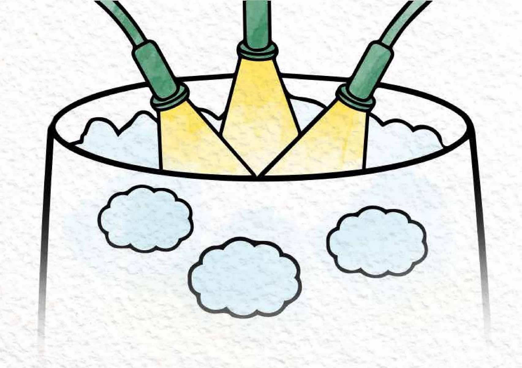
THEN THE CONCENTRATED MILK IS SPRAYED INTO A HUGE TOWER FILLED WITH HOT AIR. THE AIR IS SO HOT THAT NO HUMAN CAN GO NEAR IT.
